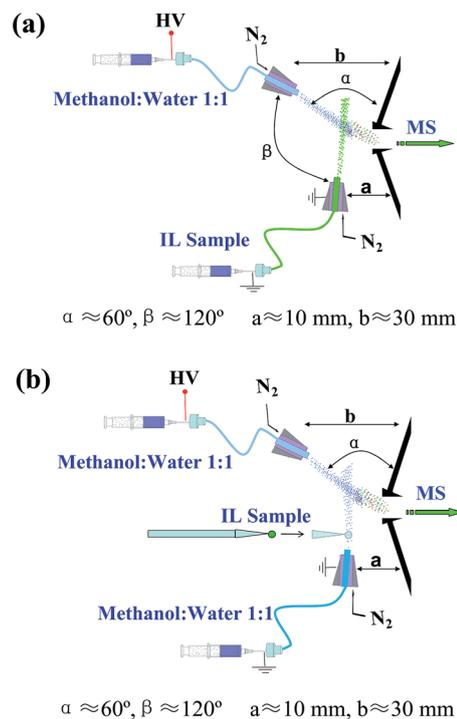
Fig. 1 Experimental configurations for the EESI-MS analysis of diluted (a) and non-diluted (b) ionic liquids.
