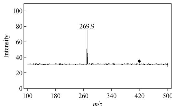
图 3  $[\text{UO}_2\text{HTar}]^+$  子离子扫描质谱图 (CID 50 V)Fig. 3 Product ions scan mass spectrum of  $[\text{UO}_2\text{HTar}]^+$  (CID 50 V)
