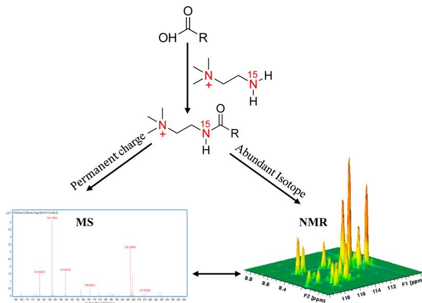
**Figure 1.** Schematic figure illustrating the “smart isotope tag” approach used to detect the same metabolites using NMR and MS with high sensitivity. Tagging carboxyl-containing metabolites with  $^{15}\text{N}$ -cholamine enables their enhanced detection by both NMR and MS.
