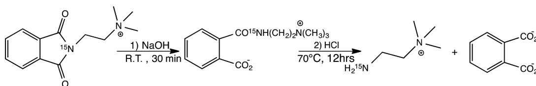
Scheme 3. General Reaction for Tagging Carboxyl-Containing Metabolites with the Smart Isotope Tag  $^{15}\text{N}$ -Cholamine
