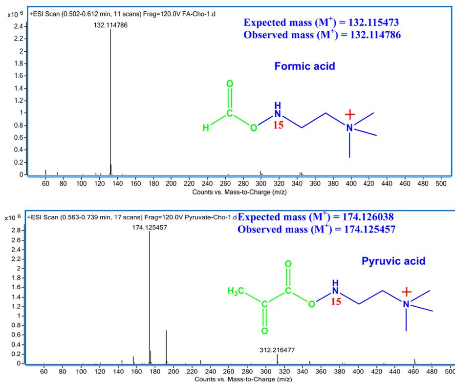
**Figure 4.** Typical LC-QTOF-MS spectra for formic acid and pyruvic acid obtained after tagging with the smart isotope tag,  $^{15}\text{N}$ -cholamine. The permanent charge on the tagged metabolites enables their sensitive detection; the observed peak is from the intact tagged metabolite.
