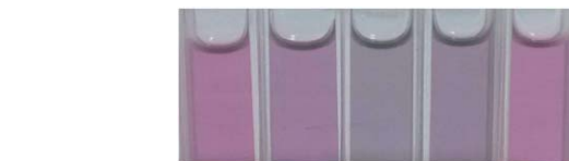
Fig. 6 The color changes of air samples above uranium ores. The air samples from left to right were control, uranium ore T-3, uranium ore 10–56, uranium ore 5–110, uranium ore H-90, respectively. 1.39 mg homemade solid reagent kit was added into each air sample.
