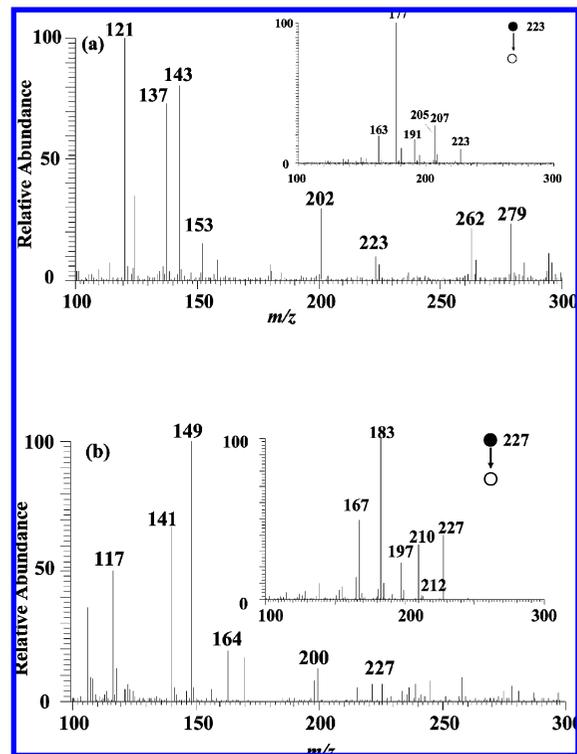
**Figure 9.** Explosives detection in groundwater using nanoEESI-MS: (a) mass spectrum of RDX in the positive ion detection mode (the inset shows the MS<sup>2</sup> of  $m/z$  223) and (b) mass spectrum of TNT in the negative ion detection mode (the inset shows the MS<sup>2</sup> of  $m/z$  227).
