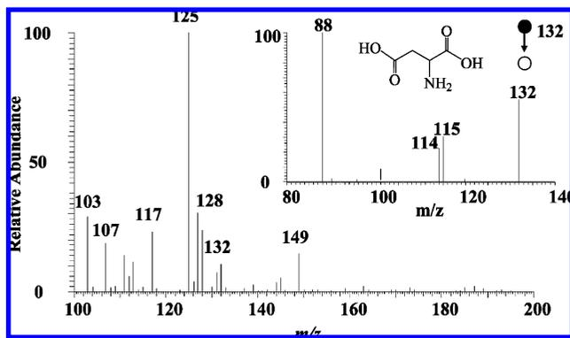
**Figure 3.** Mass spectrum of wastewater samples spiked with L-aspartic acid ( $1.0 \times 10^{-9}$  g/mL) using nanoEESI in the negative ion detection mode (inset shows the MS<sup>2</sup> spectrum of  $m/z$  132).
