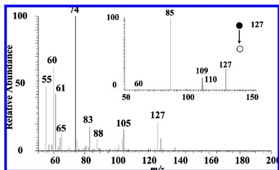
**Figure 6.** Mass spectrum of liquid milk spiked with melamine (0.2 mg/mL). The inset shows the MS<sup>2</sup> spectrum of  $m/z$  127.
