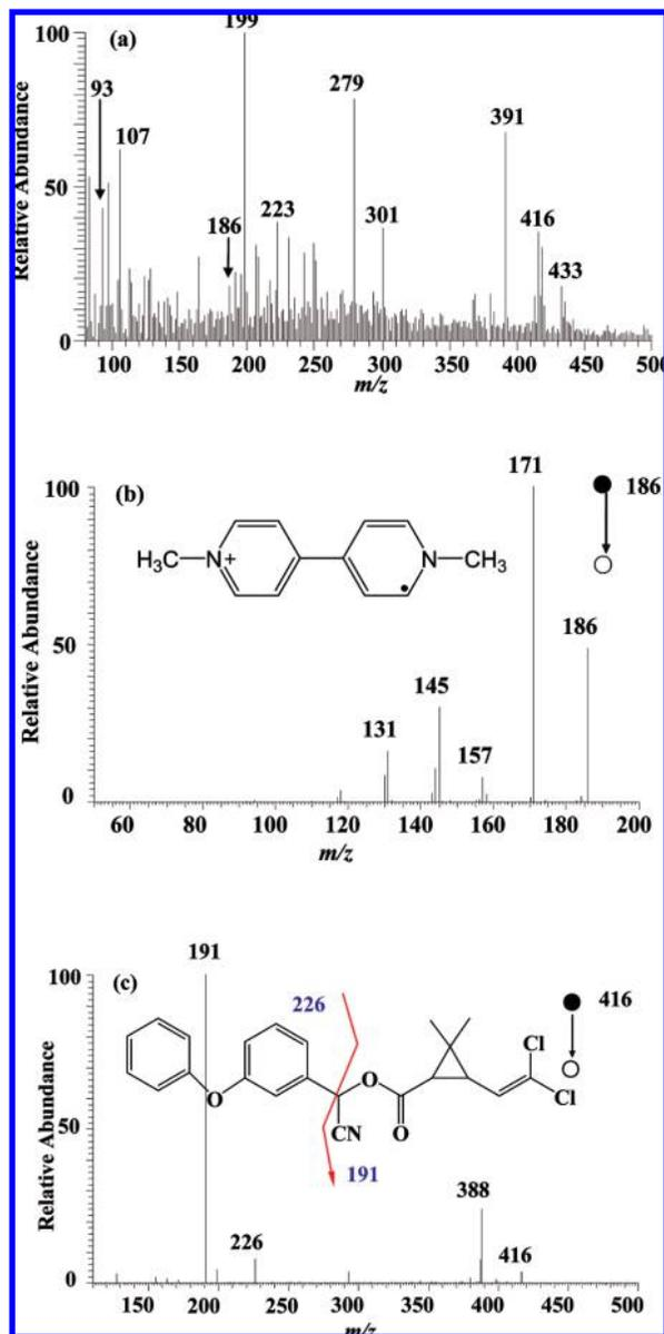
**Figure 8.** Analysis of farmland water spiked with paraquat (200 ng/mL) and  $\beta$ -cypermethrin (45 ng/mL) using nanoEESI in the positive ion detection mode: (a) full scan mass spectrum of the farmland water sample, (b) MS<sup>2</sup> spectrum of  $m/z$  186, and (c) MS<sup>2</sup> spectrum of  $m/z$  416.
