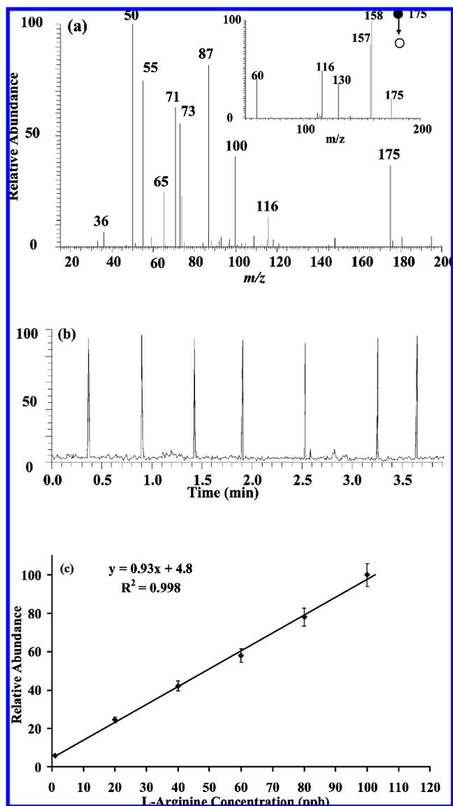
**Figure 2.** Analysis of waste water samples spiked with L-arginine using nanoEESI in the positive ion mode: (a) a full scan nanoEESI mass spectrum (inset shows  $MS^2$  spectrum of  $m/z$  175), (b) single ion chromatogram of  $m/z$  175, and (c) plot of the relative mass spectrometric abundance of protonated arginine ( $m/z$  175) vs concentration, showing the linear dynamic range between 1 and 100 ppb; the error bars designate the 5% of the mean values.
