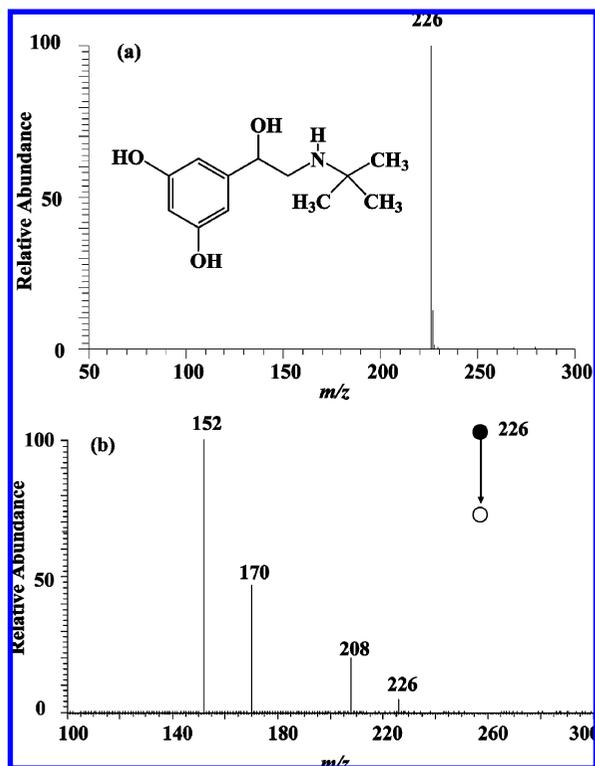
**Figure 5.** Analysis of tertbutaline aerosol drug preparations using nanoESI in the positive ion detection mode: (a) mass spectrum of tertbutaline aerosol and (b) MS<sup>2</sup> spectrum of protonated tertbutaline.
