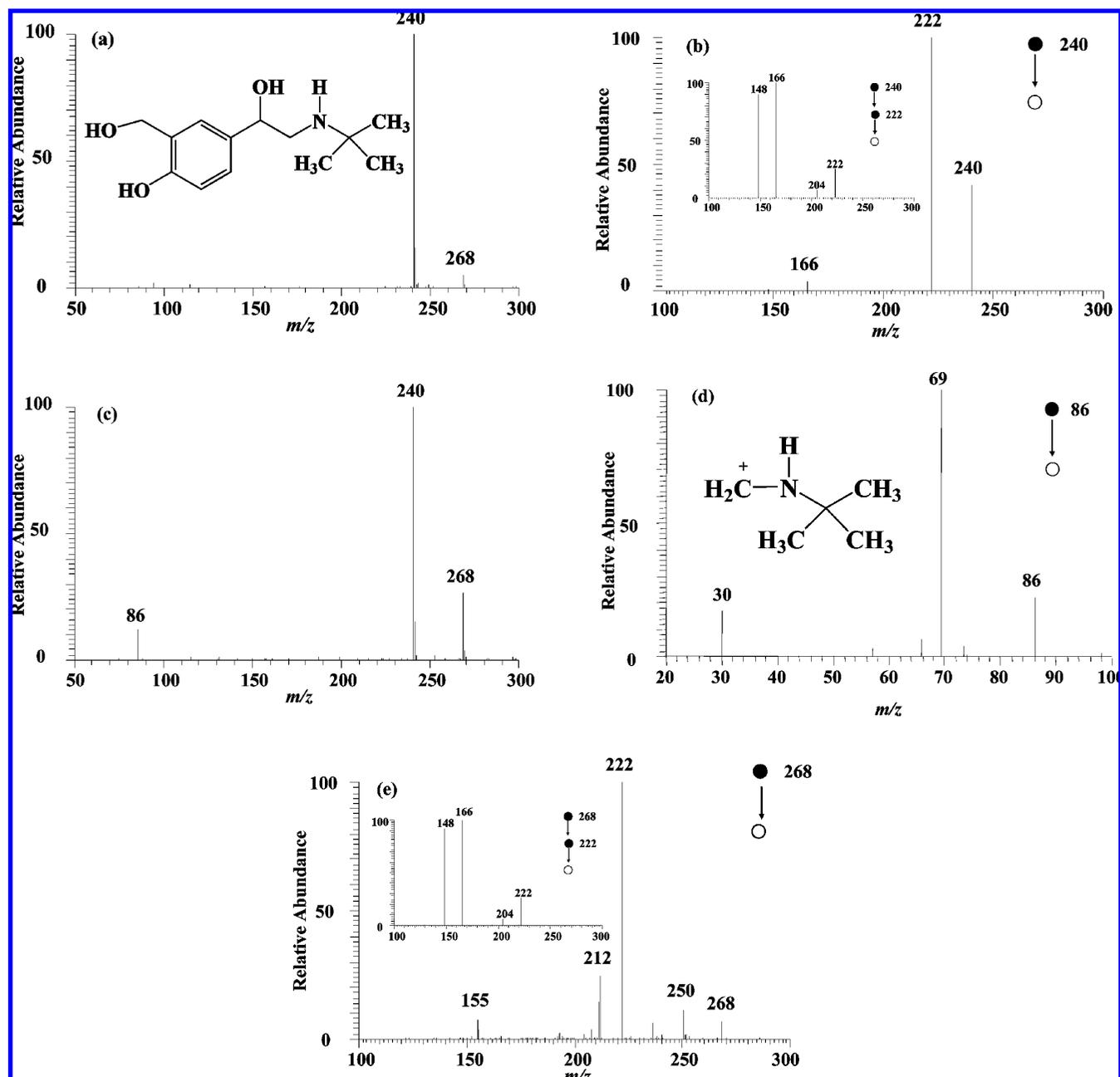
**Figure 4.** Analysis of sulbutamol aerosol drug preparations using nanoEESI in the positive ion detection mode: (a) full scan mass spectrum of sulbutamol aerosol, (b) MS<sup>2</sup> spectrum of protonated sulbutamol (inset shows the MS<sup>3</sup> spectrum of *m/z* 222), (c) mass spectrum of heat-induced expired sulbutamol, (d) MS<sup>2</sup> spectrum of the pyrolysis product (*m/z* 86), and (e) MS<sup>2</sup> spectrum of *m/z* 268 (inset shows the MS<sup>3</sup> spectrum of *m/z* 222).
