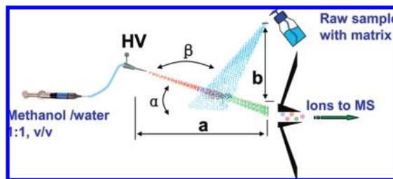
**Figure 1.** Schematic diagram of the nanoEESI source. The schematic is not proportionally scaled.
