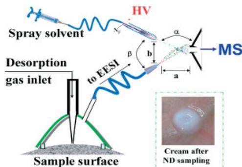
**Figure 1.** The scheme of the GIND-EESI with a sealable GIND device. The inset shows the picture of the cream on a skin surface sampled by the GIND device.
