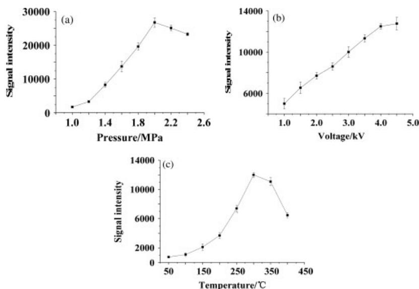
**Figure 2.** Optimization of GIND-EESI working conditions. (a) Effects of nitrogen gas pressure for ND on the EESI-MS signal intensity. (b) Effects of electrospray voltage on the EESI-MS signal intensity. (c) Effects of temperature of the ion transfer capillary on the EESI-MS signal intensity.
